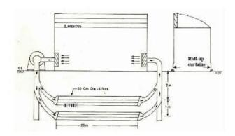
an alternative design of greenhouse technology which combines both Earth Tube Heat Exchanger (ETHE) that uses less water and static ventilation.
